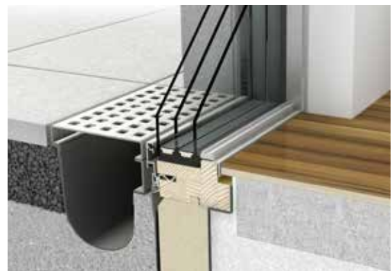
Frameless appearance and technologically optimized construction connection
