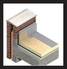
Features 125mm insulation boards to boost energy efficiency and reduce carbon emissions
